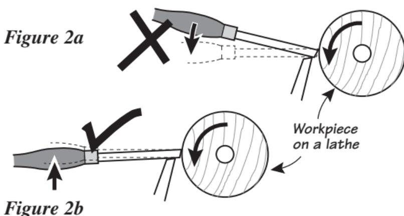
A scraper burnished with the Veritas Scraper Burnisher should be presented to the work with the bevel rubbing, then the handle lifted slightly until the tool begins to cut (**Figure 2b**). A properly sharpened scraper should produce long, continuous shavings. For end-grain work, the scraper can also be used tilted for a shearing cut.
